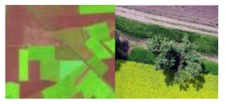
Fig. 6 Spatial resolution comparison of Satellite (LandSat 7.) and UAV based images
