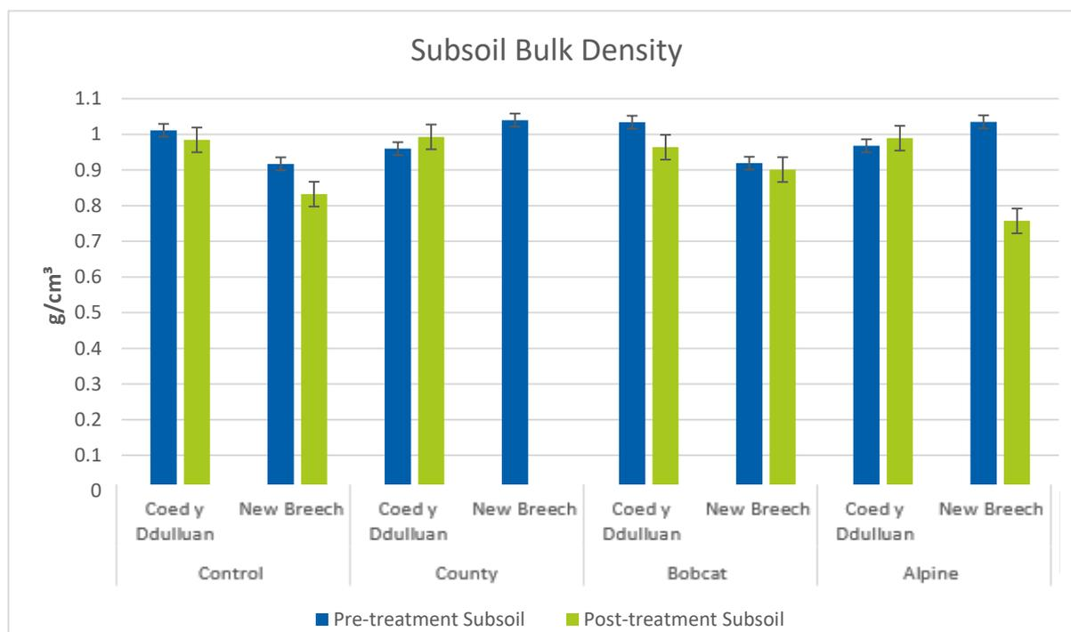
Figure 28 Post-treatment subsoil bulk density results
