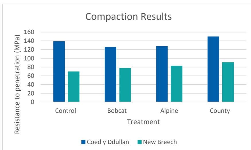
**Figure 26 Compaction results obtained from a penetrometer used in all treatment rides in Coed y Ddulluan and New Breach Wood**
