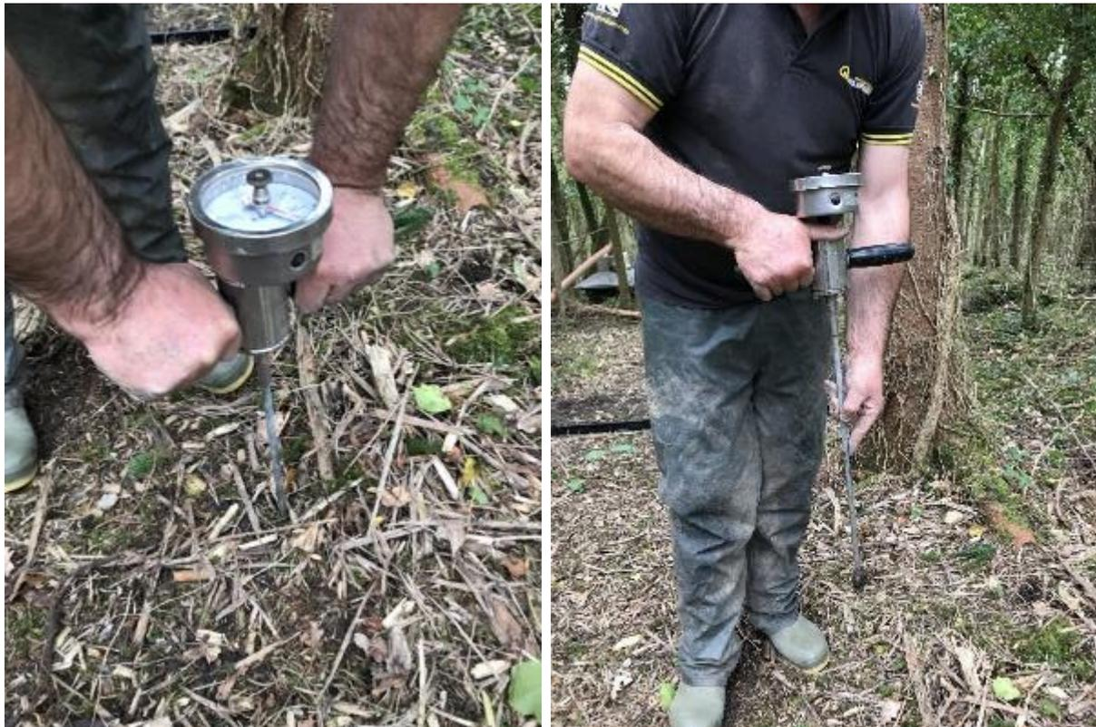
**Figure 19 Measuring for compaction using a penetrometer**
