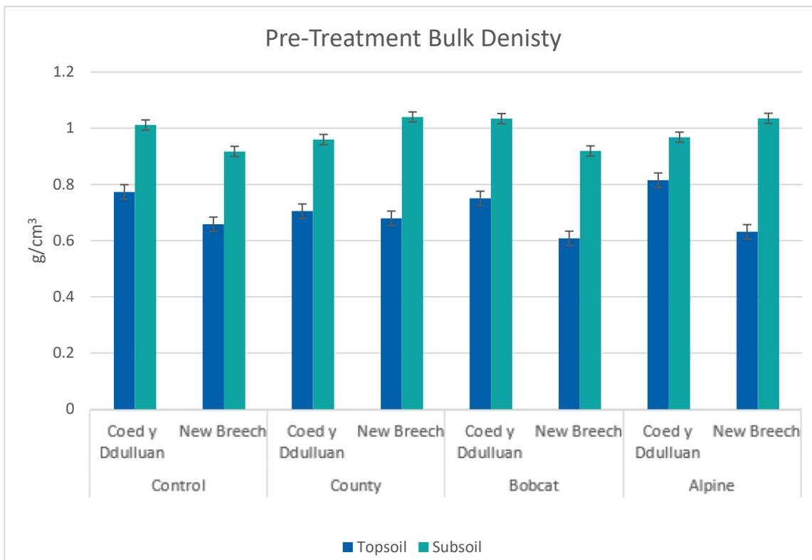
**Figure 10 Pre-treatment soil bulk density levels**
