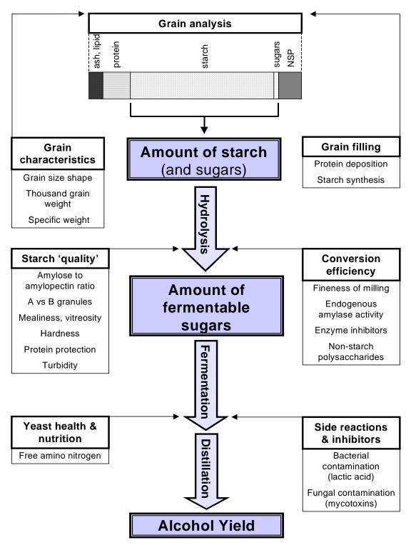
Figure 4 - Overview of the principle factors affecting alcohol processing yield and the main stages in processing at which these act.
