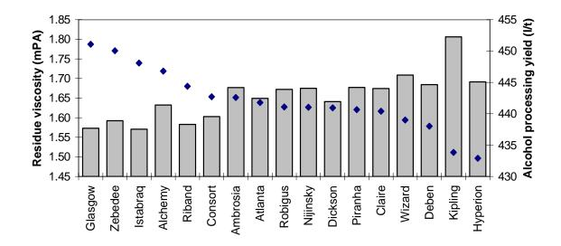
Figure 9 - Residue viscosity (mPa.s) (bars) and alcohol processing yield (l/t) (dots) measured by SWRI on varieties tested in NL and RL trials in 2003-2005 and as part of the GREEN grain project in 2005.
