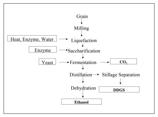
Figure 1 - Overview of the basic "dry grind" process of fuel alcohol production. The products ethanol, DDGS and  $CO_2$  are produced in approximately equal amounts by weight.
