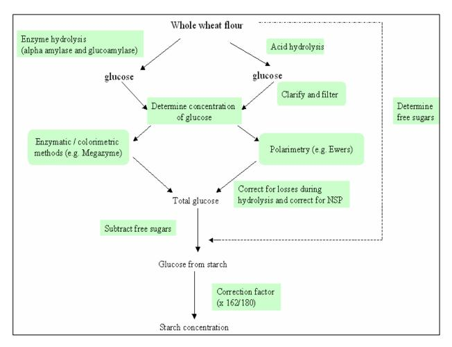
Figure 7 - Overview of the enzymatic and acid hydrolysis methods of quantifying starch.
