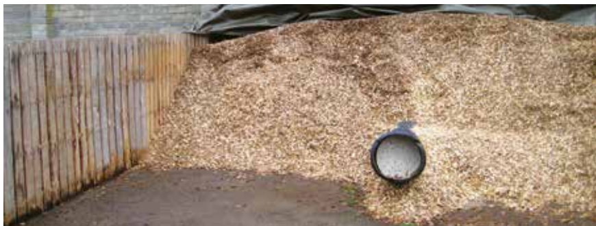
Farmyard clamp for drying willow chips
