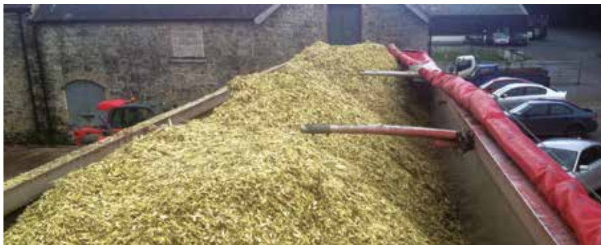
Loading a walking floor trailer with willow chips. A 100m 3 walking floor trailer will contain approx. 25 tonne of freshly harvested willow wood chip
