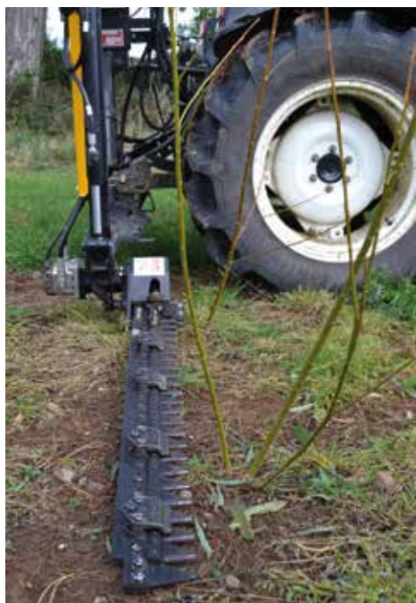
First year willow growth is cutback to within 10cm of ground level using a reciprocating type mower
