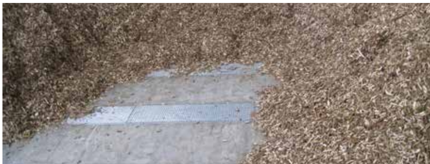
Ventilated floor drying willow chip
