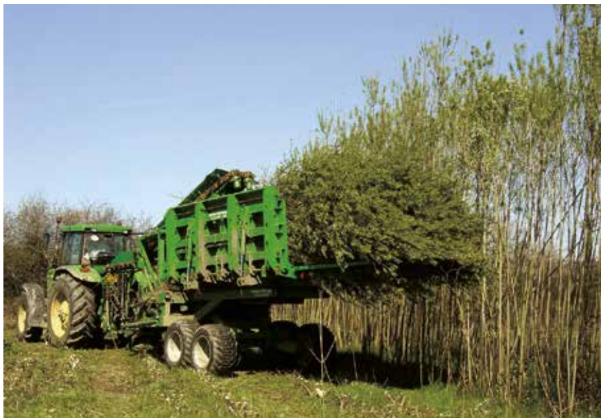
Willow being harvested with a Whole Stem harvester. Ideally harvesting should occur between December and early March when no leaves are present
